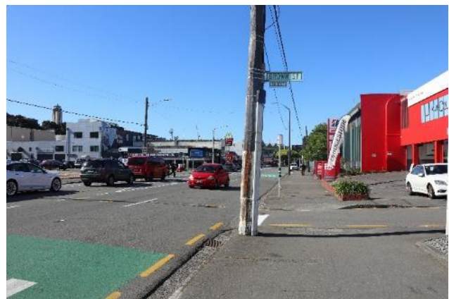
Figure 2-4: Typical view for reversing driver – intervisibility will be restricted by B Pillar of vehicle and utility poles.
