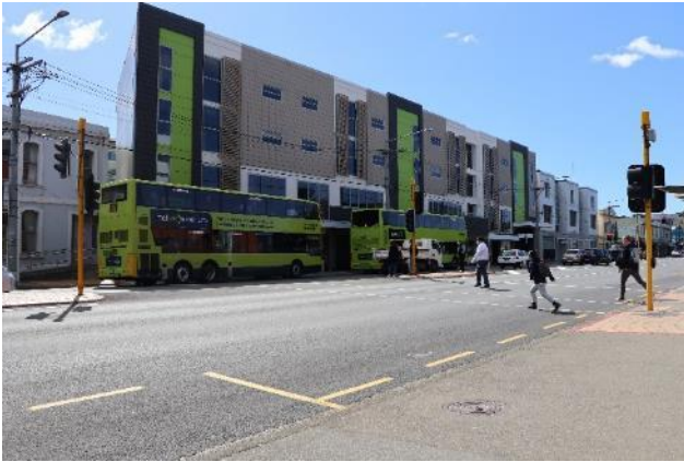
Figure 2-10: Two double deck buses at bus stop. Rear bus overhanging signalised mid-block crossing
