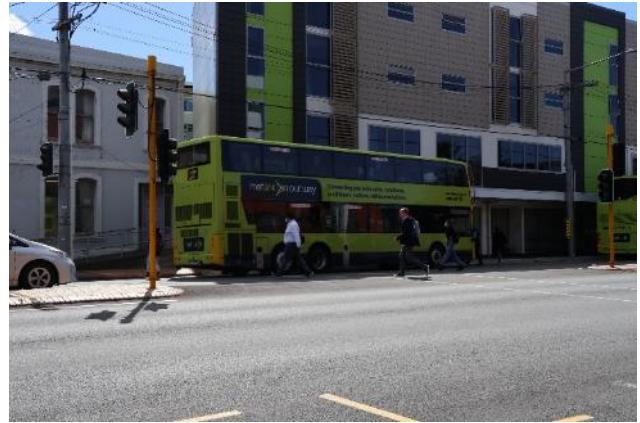
Figure 2-11: Two double deck buses at bus stop. Rear bus overhanging signalised mid-block crossing
